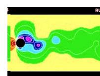
Subsonic flow around cylinder,  $Re=2000$ ,
