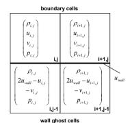
The normal momentum at a wall needs to be zero so that a wall does not apply any force onto the flow. The most simple approach, which is to simply extrapolate the pressure, is shown here.
